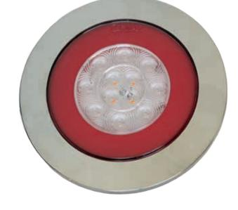
The lamp does not extend beyond the edge of the bumper - Full chassis width available for rear bumper mounting
